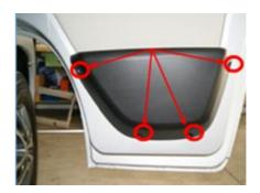
The door storage compartment must be removed in order to be able to install the door safe. In order to do so, the 4 Torx screws must be undone and removed.
